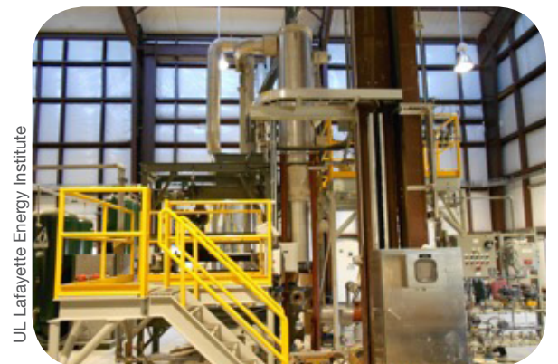
3-Ton/day Biomass fed gasifier processes wood chips to generate power and fuel. (Cleco Alternative Energy Center)
