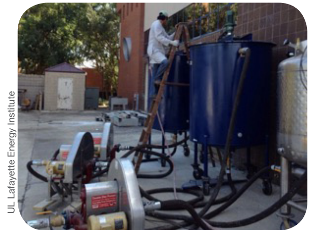
Mobile 300-gallon anaerobic digestion unit is used for researching renewable energy sources. (UL Campus)
